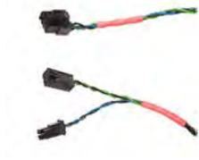
3. Connect the Controller I/O cable's 6-pin molex connector, with the black and green wires, to the laser controller socket labeled 'Analog'.
