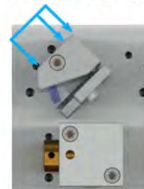
13. Use the vertical angular alignment set screw of the steering mirror to adjust the position of the beam on the pin hole vertically and maximize the power through the pin hole.
